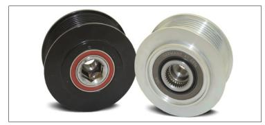
Image 1: Over-running alternator pulley 535 0214 10
